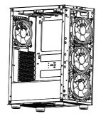
Front: 120mmx3 140mmx2 Rear: 120mmx1 Top: 120mmx2 / 140mmx2
